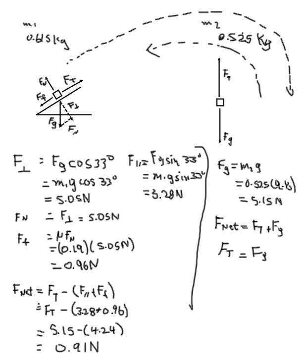
All the objects will move together as they are all connected, so we must consider the total mass of all the objects to resolve the acceleration of each object.
